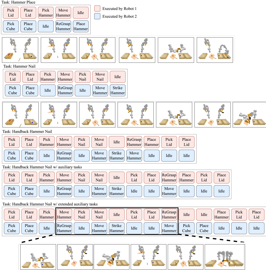
Figure S17: Extension of Hammer Nail task. We have added three new extensions to the Hammer Nail task. All of the new tasks focus on handling a second handover. The nature of the first handover adds further constraints into possible ways to perform the second handover. Further, we add task-irrelevant skills in between the plan skeleton to evaluate the robustness of GFC and the spatial-temporal factor graph plan representation.
